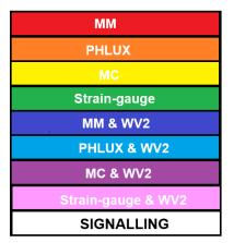
The left-hand front panel multicolour indicator indicates the input and output (I/O) options fitted in the **PHLUX-AI** preamplifier, according to the table (left).
