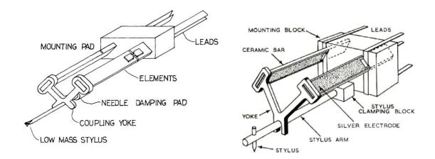
As with ceramic cartridges, the solution is a lever system as illustrated above (left – *strain-gauge*: right – *ceramic*).<sup>17,18</sup> But it's a major mechanical engineering challenge to design a phono cartridge in which the stylus ultimately pushes and pulls upon a mass reactance.<sup>19</sup>
