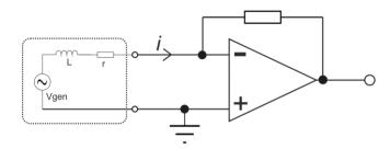
With careful electronic design, the result is a line-level voltage generated at the output of the amplifier stage which is an extremely accurate representation of the groove displacement.
