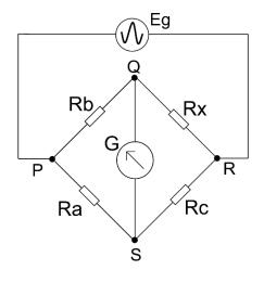
In about 1843, Sir Charles Wheatstone designed a circuit called a *bridge* which gave an accurate method for measuring *resistance*. The circuit is given left. In this circuit, resistors *Ra*, *Rb*, *Rc*, are all known values. *Rx* is the unknown resistance.
