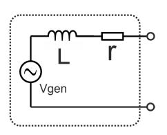
The simplified equivalent circuit of the electrodynamic pickup is given, in which a voltage generator feeds a complex internal impedance comprising a resistive component (*r*) and an inductive component (*L*). Of course, these components are not discrete and, in a stereo pickup, two such circuits exist.
