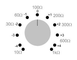
It is widely believed that input loading adjustment is worthwhile for moving-coil cartridges. To that end, when the **PHLUX-AI** preamplifier has the moving-coil front-end fitted, the bridge-balance knob controls the effect of the input loading on the cartridge by adjusting the mirror internal impedance of the Maxwell bridge.
