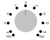
Set up the equipment and play a disc you know well, monitoring via the internal RIAA or iLOOP outputs. Select the control's central, 12 o'clock, position. If the sound is a little "lean" (bass light), rotate the balance control clockwise until you achieve the best tonal balance. If the sound balance is a little "rich" (bass heavy), rotate the control anticlockwise until you achieve the best tonal balance.
