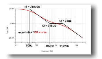
The specification of the RIAA tone-control was standardised for all records from 1955: the parameters are illustrated in the graph.
