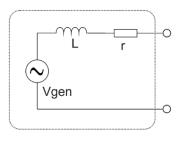
Normal operation of the electrodynamic cartridge is that the opencircuit voltage is developed across a resistor which is substantially greater in value than the resistive component of the pickup (r). It is this voltage signal which is normally amplified by the RIAA preamplifier.
